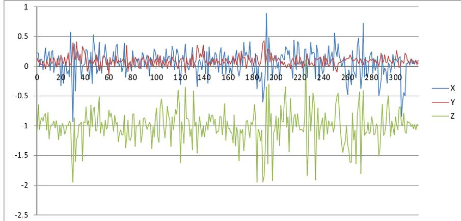
**Figure 5.** Accelerometer Data (Front, No shock absorber)
