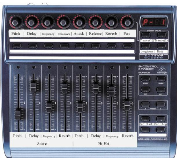
Figure 1. Controller mapping of encoders with parameters of SYNTH-WERK
