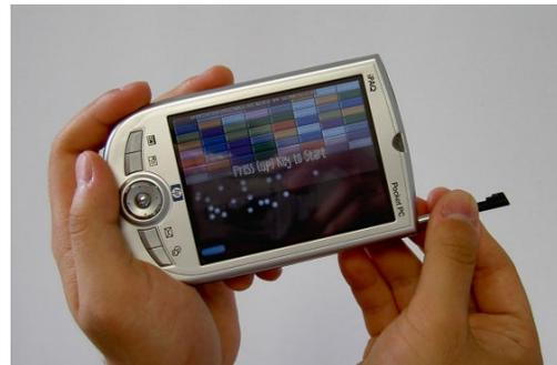
Figure 1: An interaction style of RodDirect; A user rotates and slides the stylus to operate handhelds.
